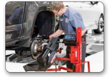
**On-Car Brake Lathe** Service each rotor precisely in less than 9 minutes.
